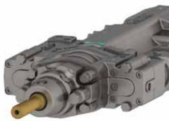
2M option replaces the gear box with two rotation motor version. It can be attached to the Doofor DF540L, DF550L and DF560L rock drills. The option improves the performance of the rock drill by increasing rotation torque.
